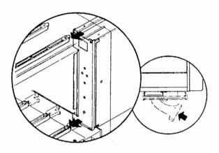
Ground the instrument to a ground terminal using a ground lead supplied as accessory. Avoid using a water pipe as a ground terminal,
