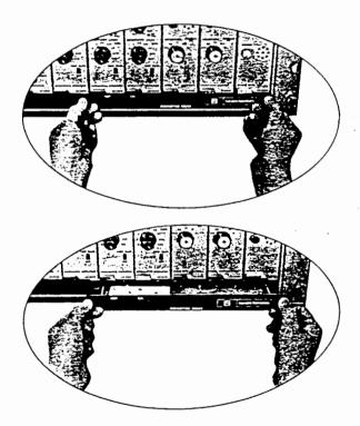
• To mount the connection board onto the console, insert the board into the console and press the two plastic buttons to fix it.
