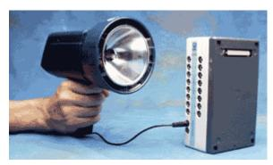
The TSD122 Stroboscope connects directly to the UIM100C or STM100C for Visual Evoked Response applications. This battery-operated device will provide 360,000 flashes between charges. The unit will go from zero to a maximum of 12,000 flashes per minute. It has external TTL synchronization and Trigger facilities for interfacing with the MP System and other equipment.
