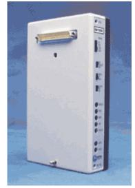
The differential amplifier module (DA100C) is a general purpose, single channel, differential amplifier. The DA100C is designed for use in the following measurement applications:
