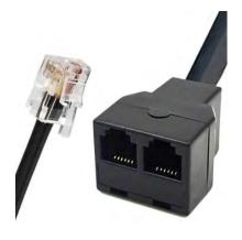
The Smart Amp Output "Y" Adapter allows for the signals from a 100D-Series Smart Amplifier connected to either an AMI100D or an IPS100D to be sent to other equipment. An RJ12 cable plugs into either the AMI100D or IPS100D, the Smart Amplifier to one port of the adapter, and either an OUTISOA for connecting signals to mains powered equipment or another cable if Unisolated connections are needed (such as CBL123).
