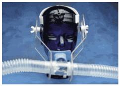
The AFT24 is a head support when breathing directly into the AFT21 non-rebreathing T valve for exercise physiology measurements. The AFT21 is secured directly in front of the subject and minimizes the strain associated with the weight of valves and tubing.
